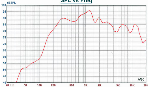
Fig. 3 - SPL at 1W/1m
