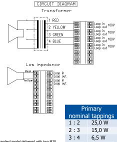
Standard model delivered with two M20 Ex approved plastic blinding plugs.
